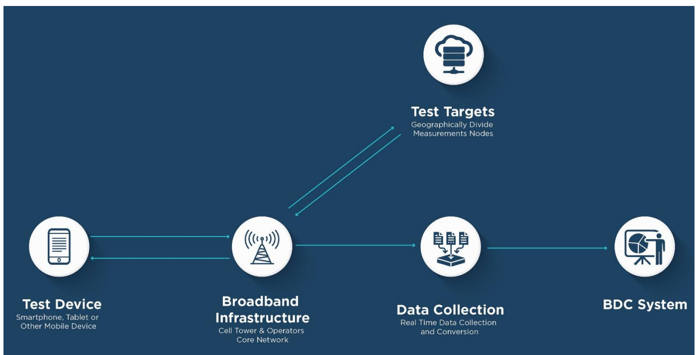
Figure 2: Mobile Broadband Test Architecture
