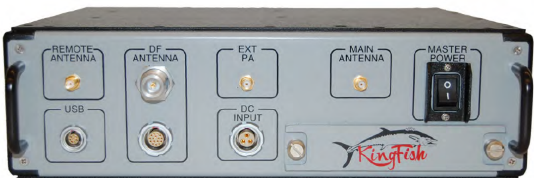
Figure 4-1. KingFish Front Panel
